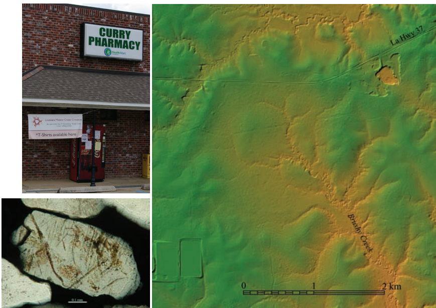
Brushy Creek LIDAR – Colored relief map of Brushy Creek crater. Created with Global Mapper 10.3 using LIDAR (Light Detection and Ranging) digital elevation model (DEM) of the southwest quarter of the Greensburg 7.5-minute quadrangle. LIDAR data downloaded from the Atlas: The Louisiana Statewide GIS website at http://atlas.lsu.edu .
