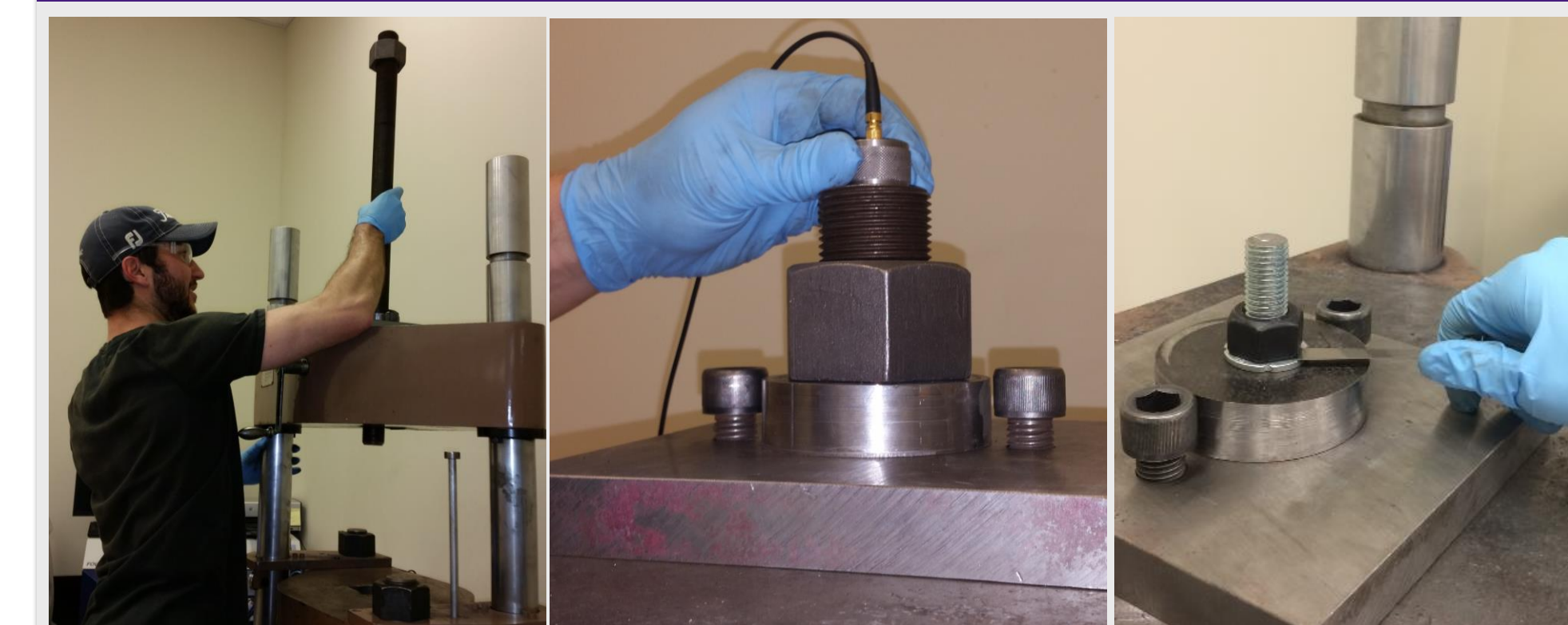
Installing 1 7/8" stud Applying transducer to 1 7/8" stud Testing Standard DTI Washers
