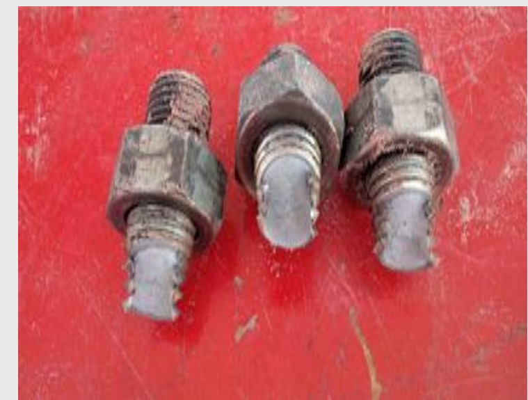
Bolt failure due to improper preload
