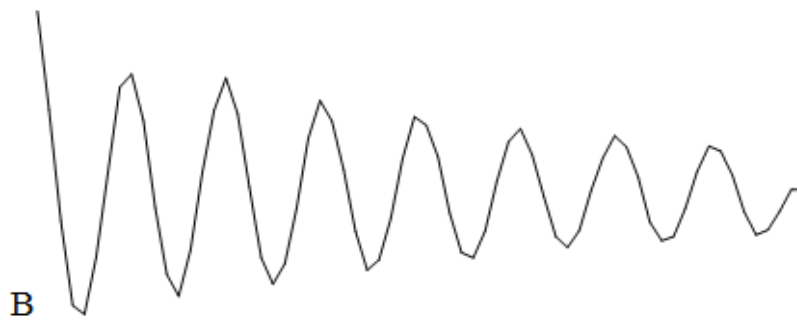
Figure 15.2: PISEMA Spectrum of 15 N Labeled Acetylated Valine and FID in t_1 over 3.008 ms 64 Data Points
