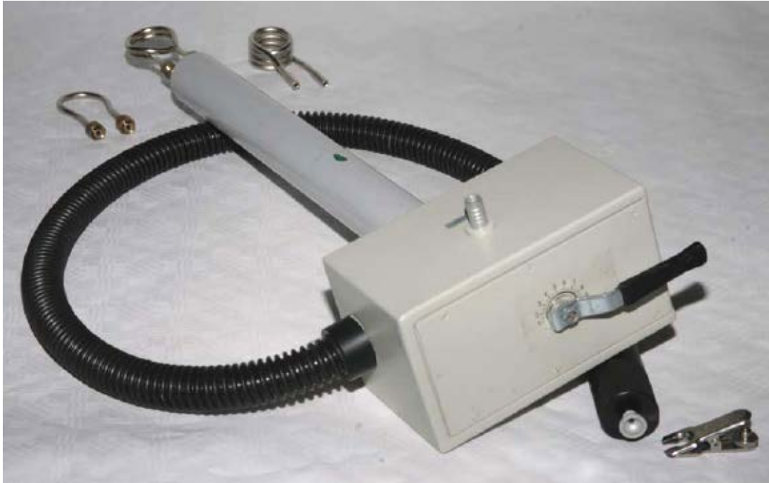
Figure 3.27: Low Temperature Heat Exchanger for VTN Probes (old style)
