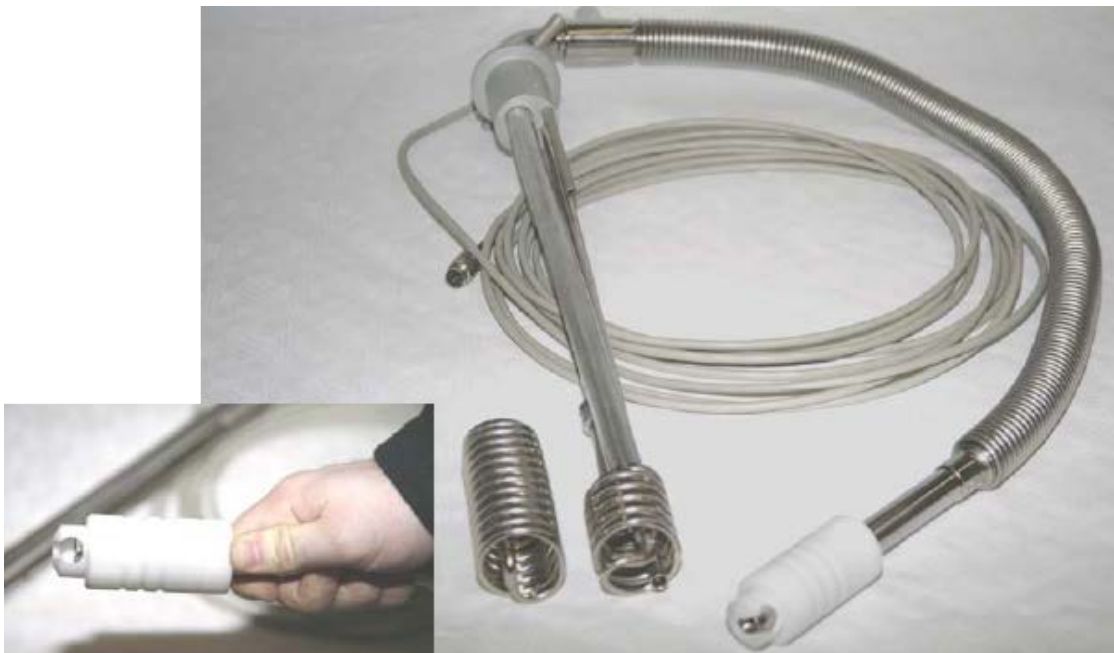
Figure 3.28: Low Temperature Heat Exchanger for DVT Probes
